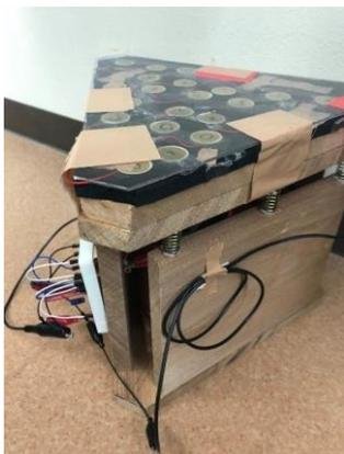
**Fig.6** Power generator used electromagnetic induction and piezoelectric elements.
