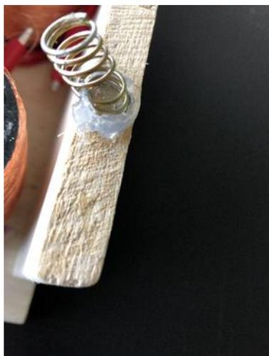
**Fig.8** Picture of damage to the spring after the trial.
