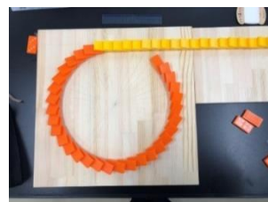
Fig. 8 Photograph of the domino falling on the curve
