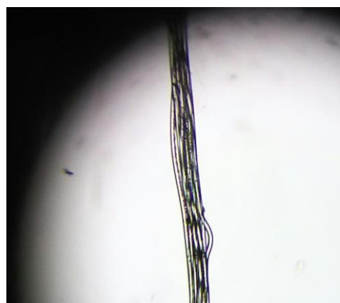
Fig.8 Structure of spider thread 倍率 15x10 倍 (顕微鏡)
